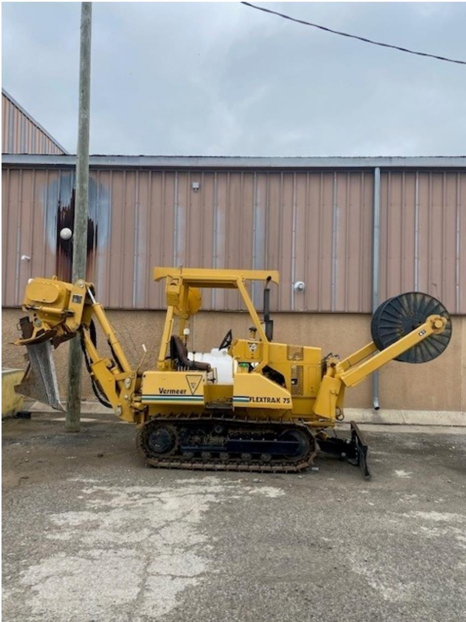
Figure 2. Bulldozer, mole plow, and cable reel.
