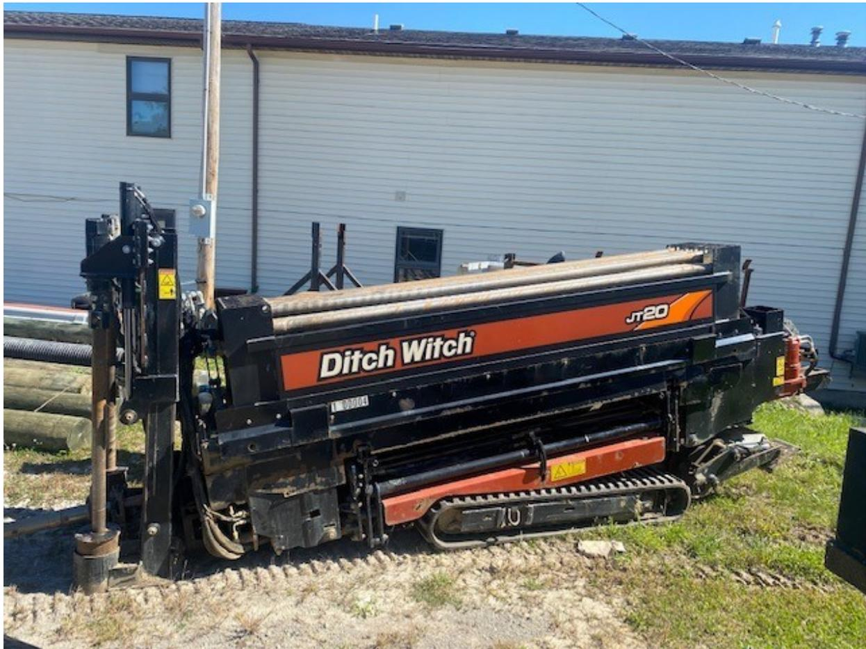
Figure 3. Directional boring machine.
